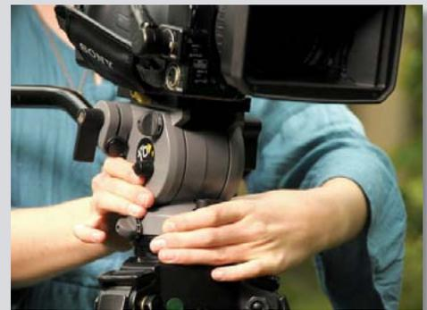
*Grip both hands around the collar of the tripod head to turn the camera*
